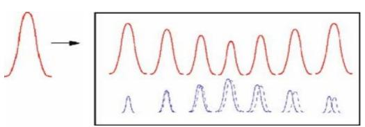
Fig. 3 Illustration of FF and SH pulses propagating in a quadratic nonlinear crystal. The dashed lines represent the propagation in the absence of GVM
