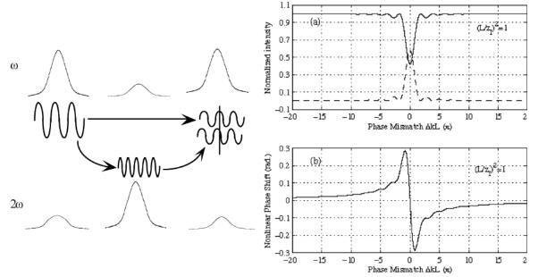
Fig. 1 Left panel: Origin of the cascaded quadratic phase shift. Some of the fundamental ield undergoes one or more cycles of conversion and back-conversion. When the energy
