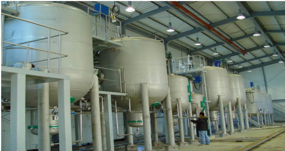
Fig. 27: To cultivate the adventitious roots of ginseng, large-scale (10,000l) bioreactors were created. Source-www.merkmillipore.com
