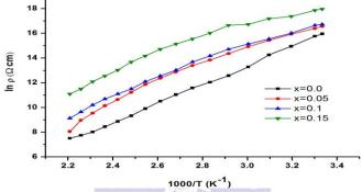
Figure 6 : Compositional variation of DC resistivity of CoFe<sub>2-x</sub>NdxO<sub>4</sub> with inverse temperature
