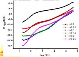
conduction is the result of minor polaron hopping. Small polaron formation may result from oxygen vacancies or defect levels introduced during sintering. The Frequency Dependence of Ac can Be Elucidated Using the Two-Layer Model of Polycrystalline Ferrites by Maxwell and Wagner.
