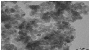
Figure 3(a) The Distribution of Cofe204 Nanoparticles
