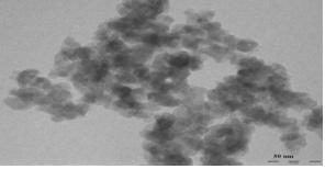
Figure 2(a) TEM image of CoFe<sub>2</sub>O<sub>4</sub>
