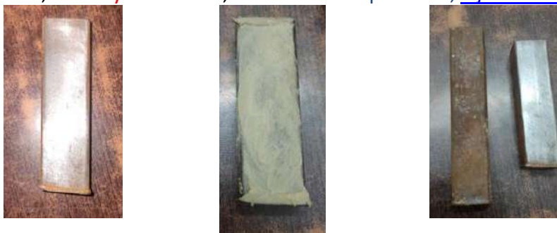
Normal Iron After coating of grease Effect of greaese
